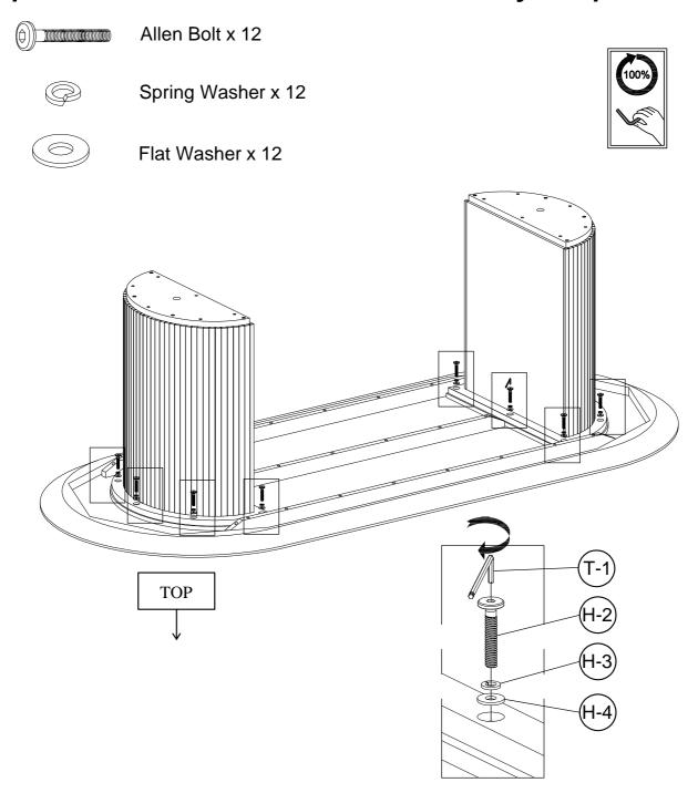
Secure Table Top (A) to the Leg Frame (B) using Allen Bolts (H-2), Spring Washers (H-3) and Flat Washers (H-4), stacking the hardware in the order shown. Engage all bolts by hand but do not fully tighten them yet. Once all hardware are installed, securely tighten all hardware using Allen Key (T-1).
